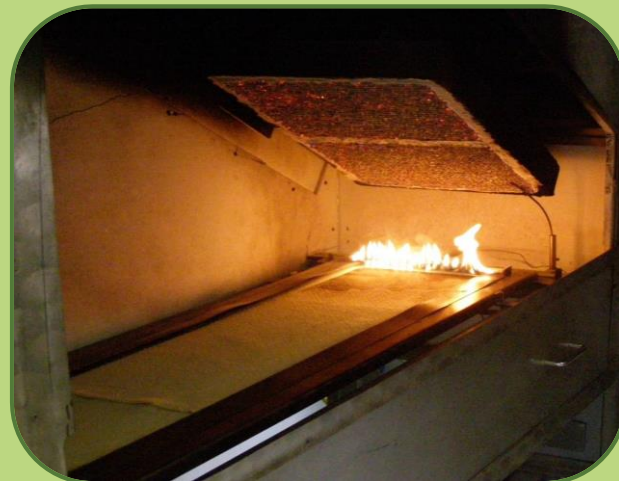
Floor radiant panel test (EN ISO 9239-1). A heat flux of 0 to 11 kW/m 2 is applied along the specimen. Our bio-coatings reached the B_{fl-s1} classification.
