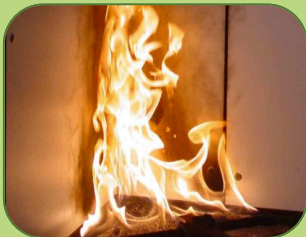
The single burning item test (EN 13823) involves applying a heat flux of 40-50 kW/m 2 to a limited area of the tested material. Our bio-coatings successfully reached B-s1, d0 classification.
