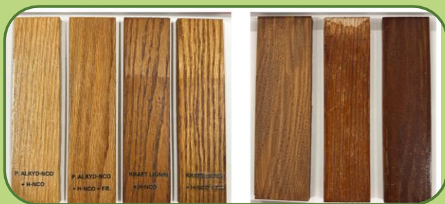
Final coatings prototypes for two target classes: flame retardant coatings reaction to fire B_{fl}-s1 (left), and intumescent coatings reaction to fire B-s1, d0 (right).
