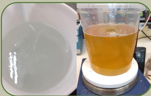
Sugar-modified resin with thymol (left) and sugar-modified resin with hop resin (right).
