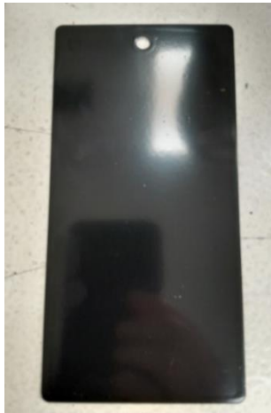
After application of biocoating by spray gun
