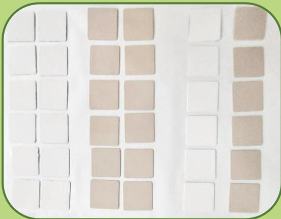
Antimicrobial efficacy test of paints based on conventional alkyd (two columns on the left) and bio-alkyd (two columns in the middle).
