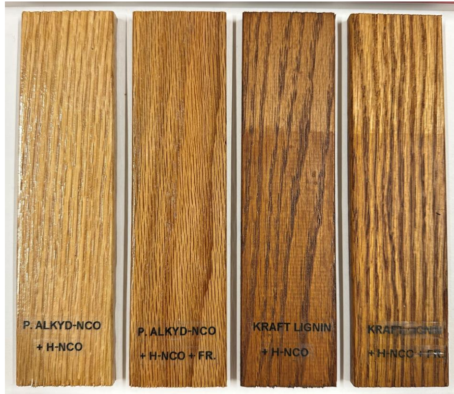
FLAME RETARDANT COATINGS reaction to fire Bfl-s1 ?
