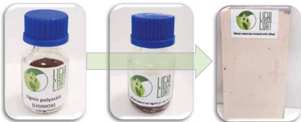
Alkyd resins on metal based on lignin polyacids
