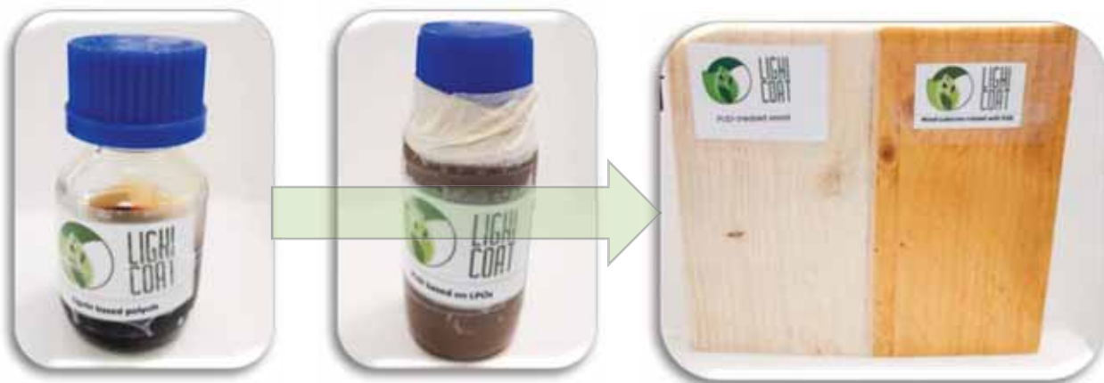
Polyurethane coating on wood based on lignin polyols
